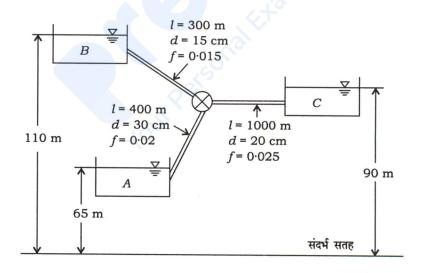
Reservoir A (elevation 65 m) is filling reservoir B (elevation 110 m) and reservoir C (elevation 90 m) by a pump and pipe system. The discharge to reservoir C is  $0.10 \text{ m}^3/\text{s}$ . If the efficiency of the pump is 0.70, calculate the required power
