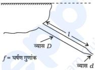
Prove that the power transmission through nozzle is maximum when  $\frac{d}{D} = \sqrt{\frac{D}{8fl}}$ . Neglect the minor losses.
