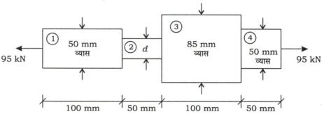
A rod shown in the figure below is subjected to a force of 95 kN. Determine the diameter d of the portion 2, if the stress there is not to exceed 115 N/mm<sup>2</sup>. Also, determine the axial deformation of the rod. Use E = 205 GPa:
