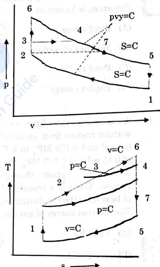
The figures show the compression of Otto, Diesel and Dual cycles for the same compression ratio and heat rejection. The Otto cycle is
