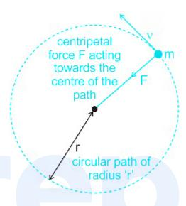
The centripetal force required for circular motion along the surface of the road, towards the center of the turn. The Static friction between tire and road provides the necessary centripetal force.
