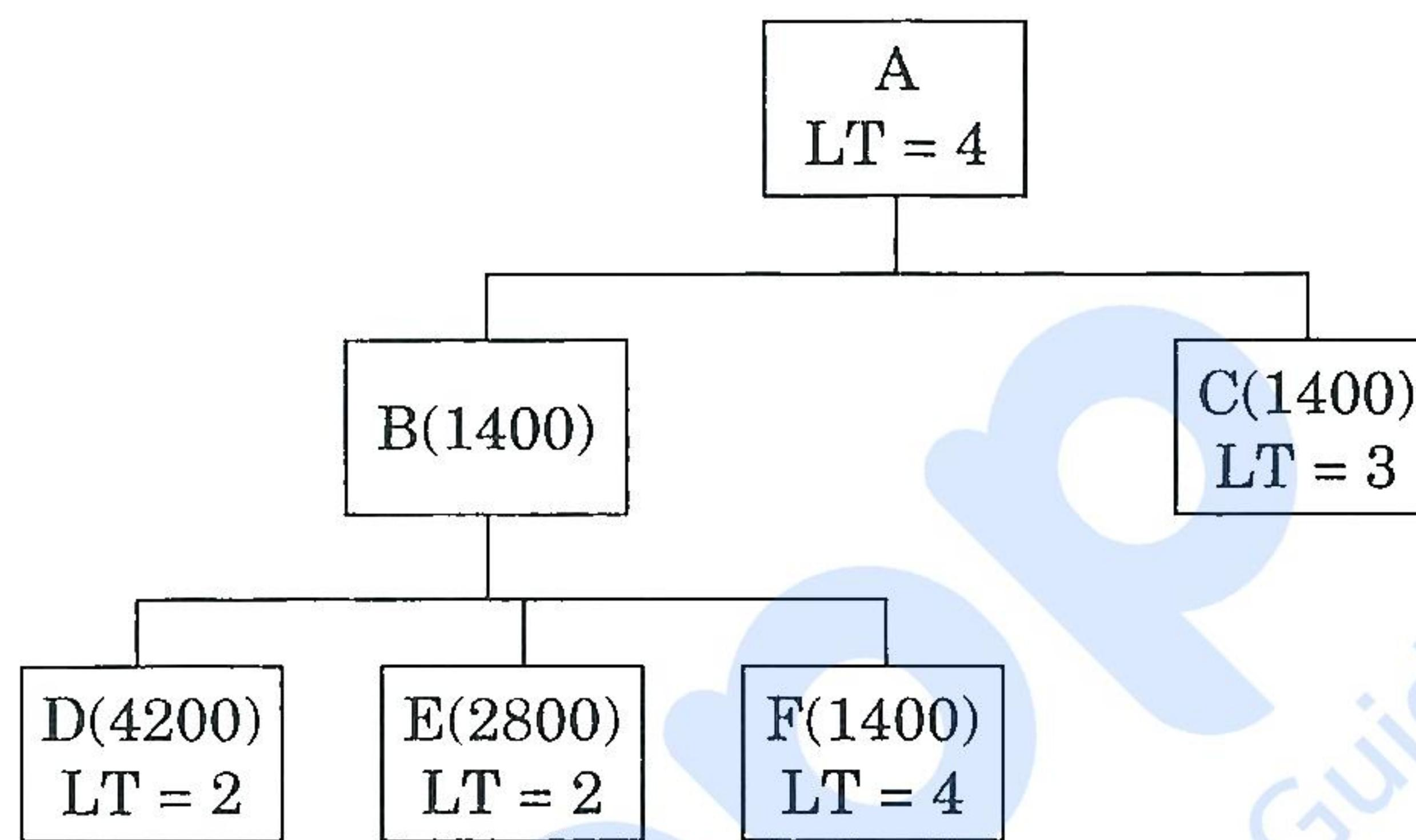
Given the following product structure of A; explode, offset and determine the gross and net requirements. All lead times (LT) are in weeks and the quantities required are shown in parentheses. The MPS calls for 700 units of product A, to be delivered in week 12. The company has in hand 300 units of each of the components C and E.
