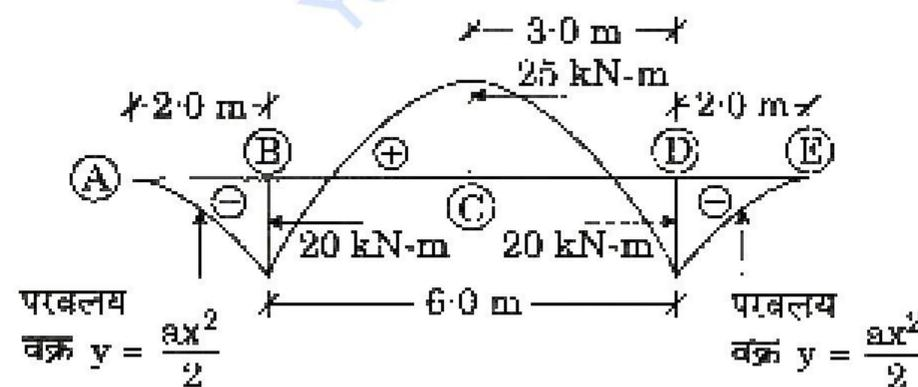
Bending moment diagram for a beam carrying uniformly distributed load has been shown below. Bending moment diagram curve is parabolic and follows the equation  $y = \frac{ax^2}{2}$  in AB and DE portion.
