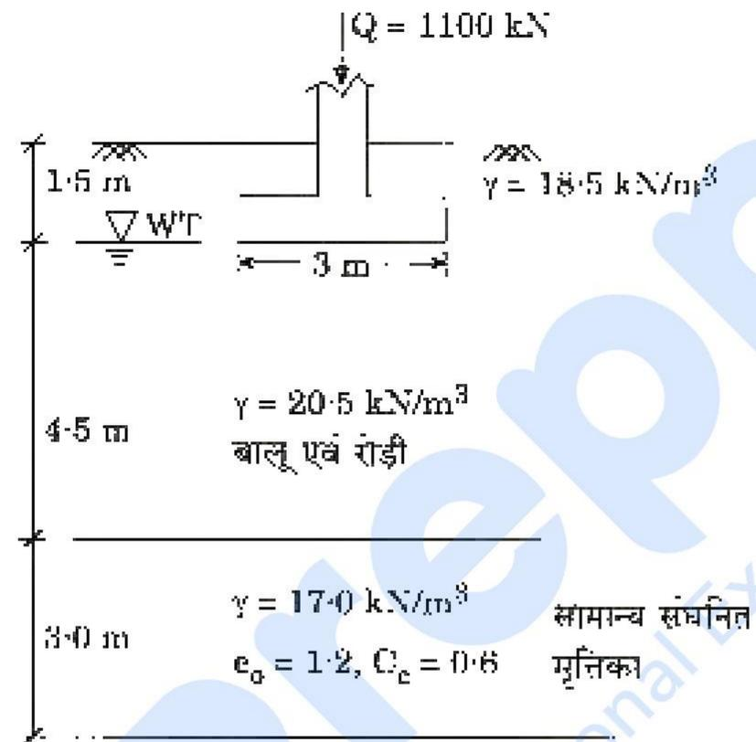
A square footing of size 3 m  $\times$  3 m is placed on a sand and gravel layer at a depth of 1.5 m from the ground surface. Below the sand and gravel layer, a layer of normally consolidated soil of thickness 3 m is present. Details of soil properties and the footing loading are shown in the figure. Determine the total expected consolidation settlement for the clay layer because of the footing loading.
