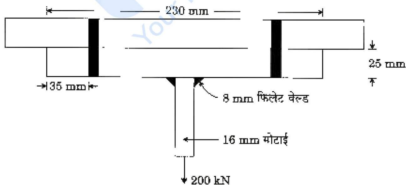
Check the adequacy of the hanger connection shown in the figure below. The end plate welded connection shown in the figure need not be designed. The end distance of the bolt is 35 mm. Two bolts of 30 mm diameter are used to make the connection. The end plate is 230 mm × 150 mm in size. For 30 mm bolt,  $A_{cb} = 561 \text{ mm}^2$ ,  $d_h$  and  $d_v = 33 \text{ mm}$ ,  $f_{yb} = 400 \text{ MPa}$ .
