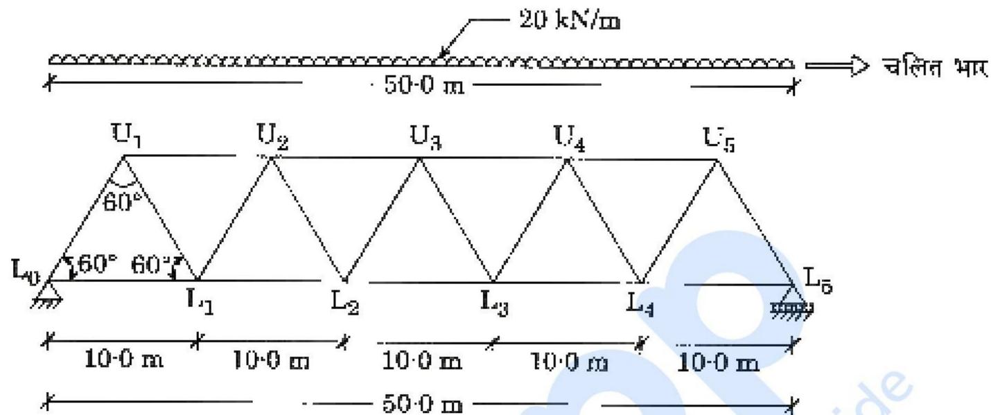
Calculate maximum force in the diagonal member  $U_2L_2$  of the truss shown in the figure below, for a moving load of 20 kN/m (intensity) and 50.0 m in length. It is proposed that this moving load will be transmitted through the bottom chord. (Neglect the self-weight of truss)
