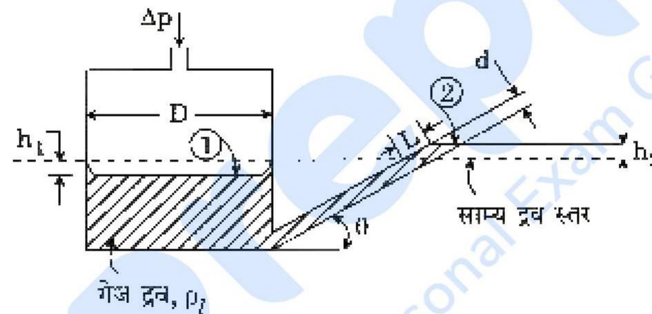
An inclined tube reservoir manometer is constructed as shown. Derive a general expression for the liquid deflection,  $L$ , in the inclined tube, due to the applied pressure difference,  $\Delta p$ .
