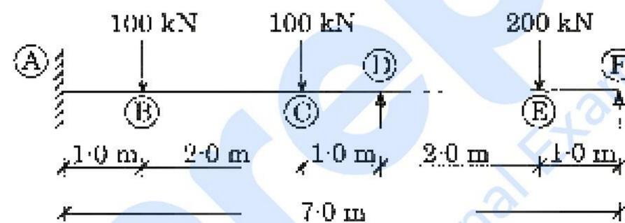
Calculate the value of Plastic Moment ' $M_p$ ' for the beam shown below.
