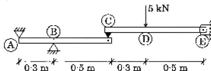
Draw the free body diagram for lower and upper parts of the system. Calculate all reactions for the figure shown below.
