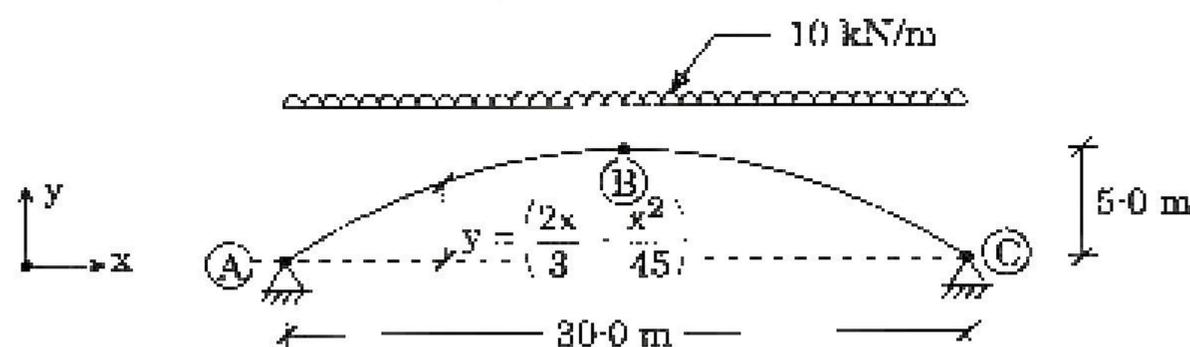
A three-hinge parabolic arch,  $y = \frac{2x}{3} - \frac{x^2}{45}$  has a span of 30.0 m and maximum rise of 5.0 m at centre. Arch is having uniform cross-section throughout. It is subjected to uniformly distributed load of 10 kN/m (dead load + live load).
