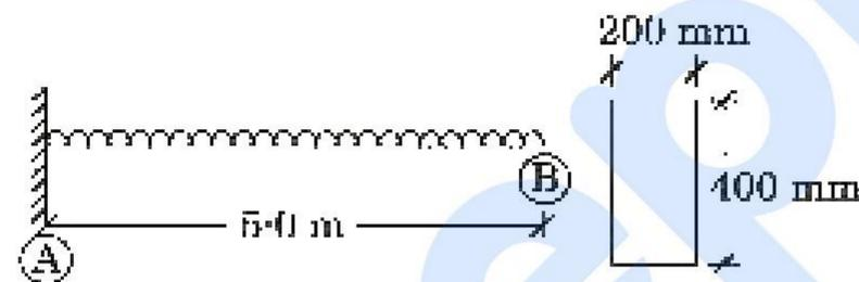
A cantilever beam carries a uniformly distributed load over its entire length. Maximum possible deflection at the free end 'B' is limited to 40 mm. Calculate the magnitude of maximum possible uniformly distributed load (dead load + live load) for a combined factor of safety of 1.5 on this beam.
