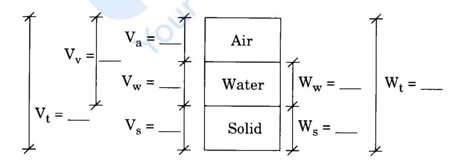
$V_t$  = total volume,  $V_v$  = volume of void,  $V_a$  = volume of air,  $V_w$  = volume of water,  $V_s$  = volume of solids,  $W_t$  = total weight,  $W_w$  = weight of water,  $W_s$  = weight of solids.
