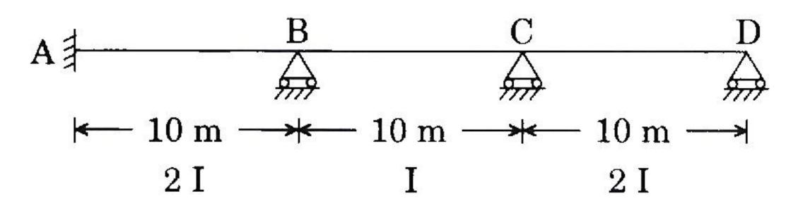
Calculate the flexural stiffness at point 'D' of the three span continuous beam ABCD shown in the figure below.
