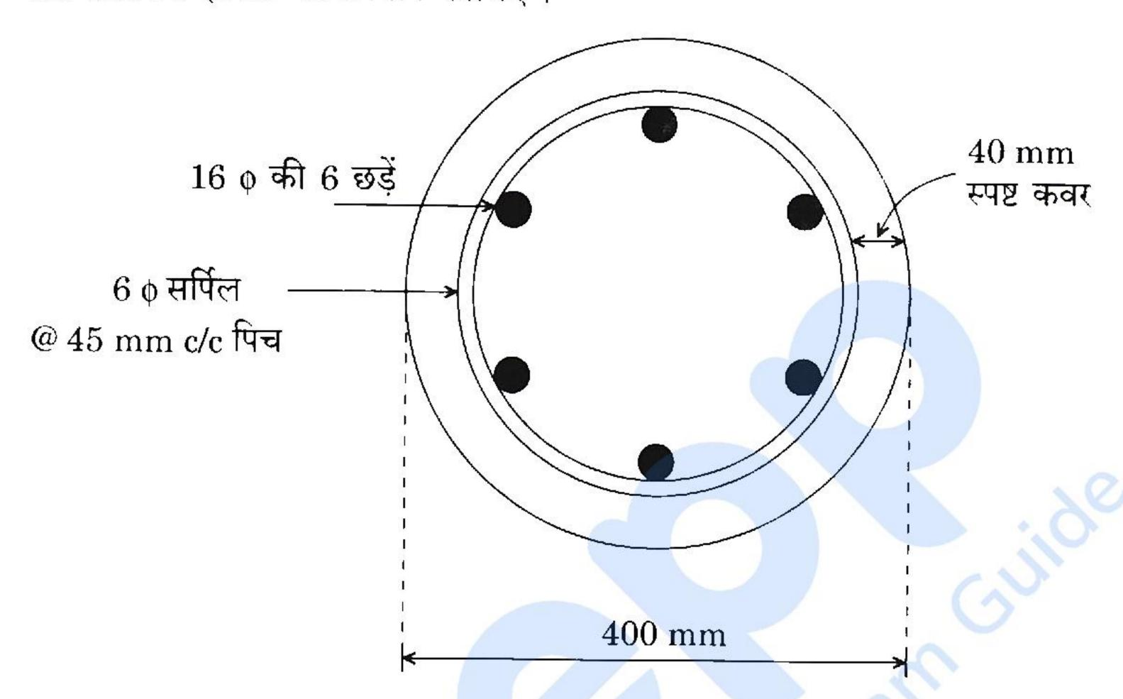
A column has an unsupported length of 3·4 m and is effectively held in position at its both ends, but not restrained against rotation. The cross-section of the column and reinforcement details are shown in the figure below. Determine the safe axial load that the column can carry. Use M 25 grade of concrete and Fe 415 grade of steel.
