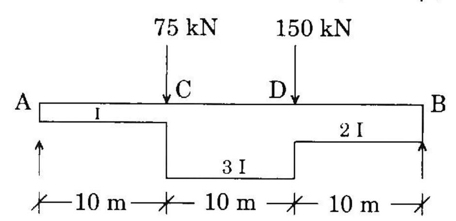
Using conjugate beam method, for the beam shown below, find the slopes and deflections at 'A', 'B', 'C' and 'D'. Given :  $E = 200 \times 10^6 \text{ kN/m}^2$  and  $I = 300 \times 10^{-4} \text{ m}^4$ . Neglect the weight of the beam.
