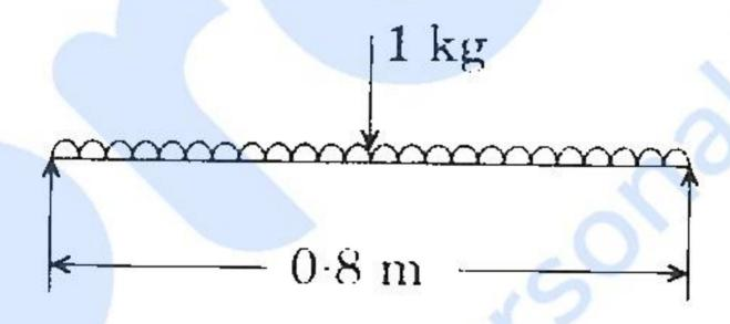
Determine the whirling speed of a shaft 25 mm diameter and 0.8 m long with a mass of 1 kg placed at mid span, simply supported at ends. The density of the shaft material is 50 g/cm<sup>3</sup> and Young's modulus is  $2 \times 10^6$  bar.
