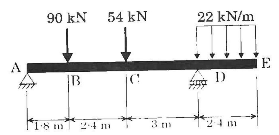
Draw the shear force and bending moment diagrams for the beam and loading shown. Also determine the maximum values of shear force and bending moment along with their respective locations.
