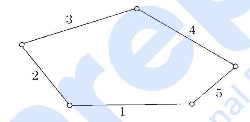
A five-bar chain is shown in the figure. Prove that it is an unconstrained chain.
