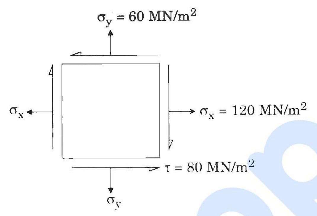
At a certain point in a piece of elastic material, there are normal tensile stresses of magnitude 120 MN/m<sup>2</sup>, 60 MN/m<sup>2</sup> acting orthogonally to each other. In addition, there is a shearing stress of 80 MN/m<sup>2</sup> acting normal to the normal stresses.
