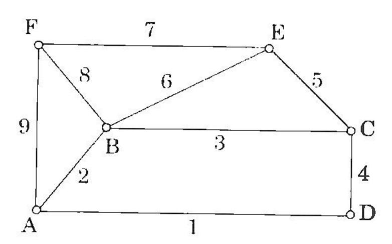
Show that the chain shown in the figure is not a kinematic chain.
