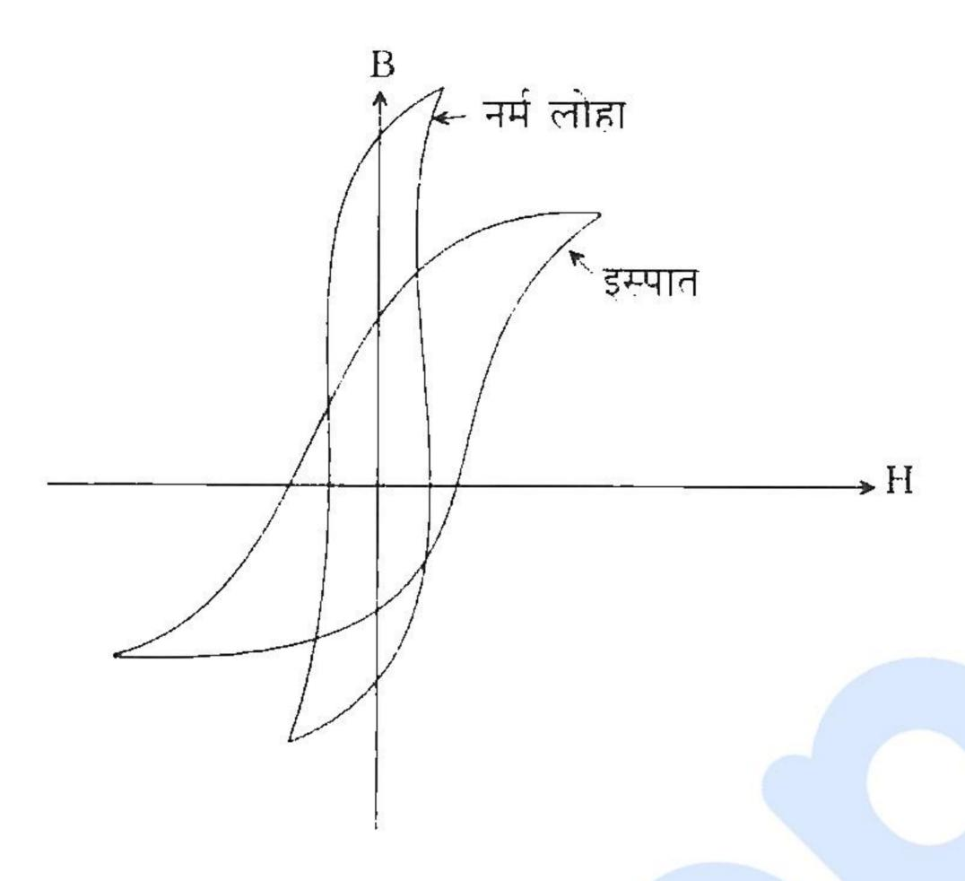
Based on the hysteresis loops for soft iron and steel as shown in the diagram, which material would you prefer to utilise for making transformer cores and why?
