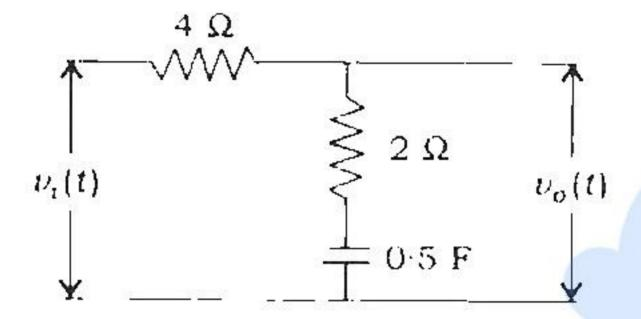
A sinusoidal voltage  $v_i(t)$  is applied to the lag network shown in the figure below.  $v_i(t)$  is adjusted to produce a sinusoidal steady-state output voltage  $v_o(t) = 2\sin(\omega t + 45^\circ)$  volts. If  $\omega = 1$  rad/sec, determine the input voltage  $v_i(t)$ .
