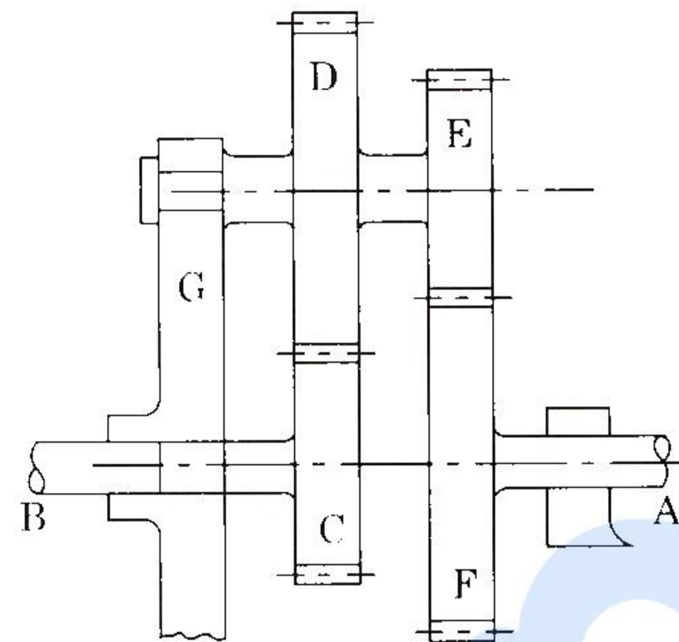
In the epicyclic gear train shown in the figure, the wheel 'C' is keyed to the shaft 'B'. 'D' and 'E' are compound gears. 'C', 'D' and 'E' have 35, 65 and 32 teeth respectively. All the gears have same module.
