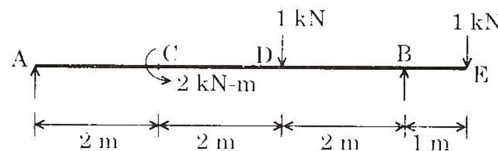
Write the equations for shearing force and bending moment for various sections and draw SFD and BMD for the beam supported at A and B as shown in the figure.
