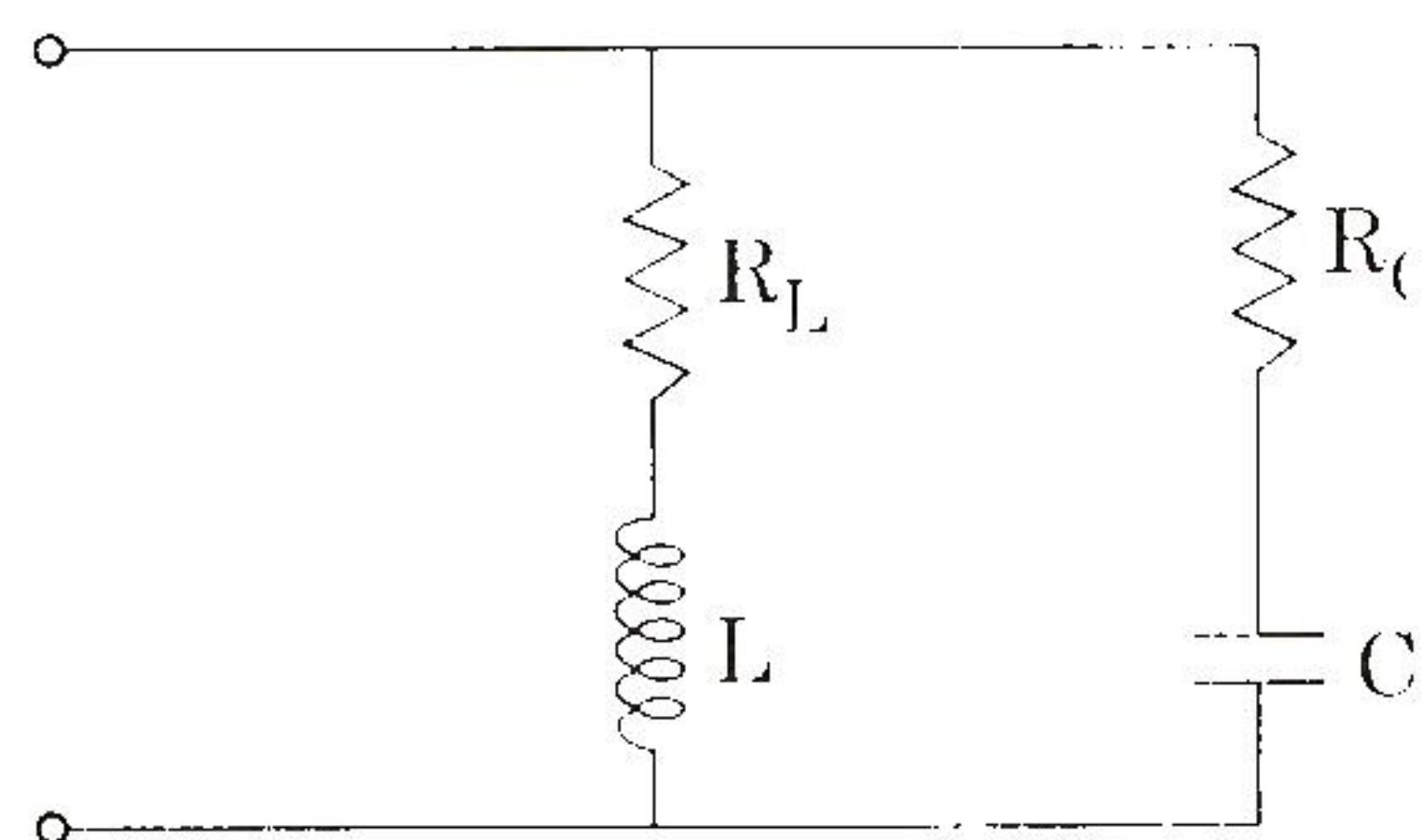
Consider the two branch parallel circuit shown in the diagram.
