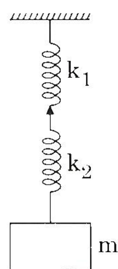
A mass  $m$  is suspended by two springs having force constants  $k_1$  and  $k_2$  as shown in the figure. The mass  $m$  is displaced vertically downward and then released. If at any instant  $t$ , the displacement of the mass  $m$  is  $x$ , then show that the motion of the mass is simple harmonic motion having frequency
