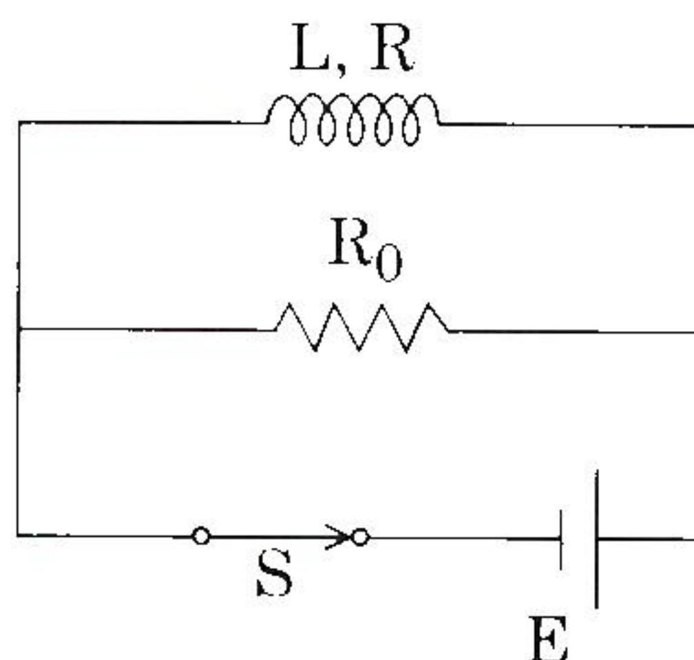
In the given circuit,  $L = 2\cdot0 \mu\text{H}$ ,  $R = 1\cdot0 \Omega$ ,  $R_0 = 2\cdot0 \Omega$  and  $E = 3\cdot0 \text{ V}$ .
