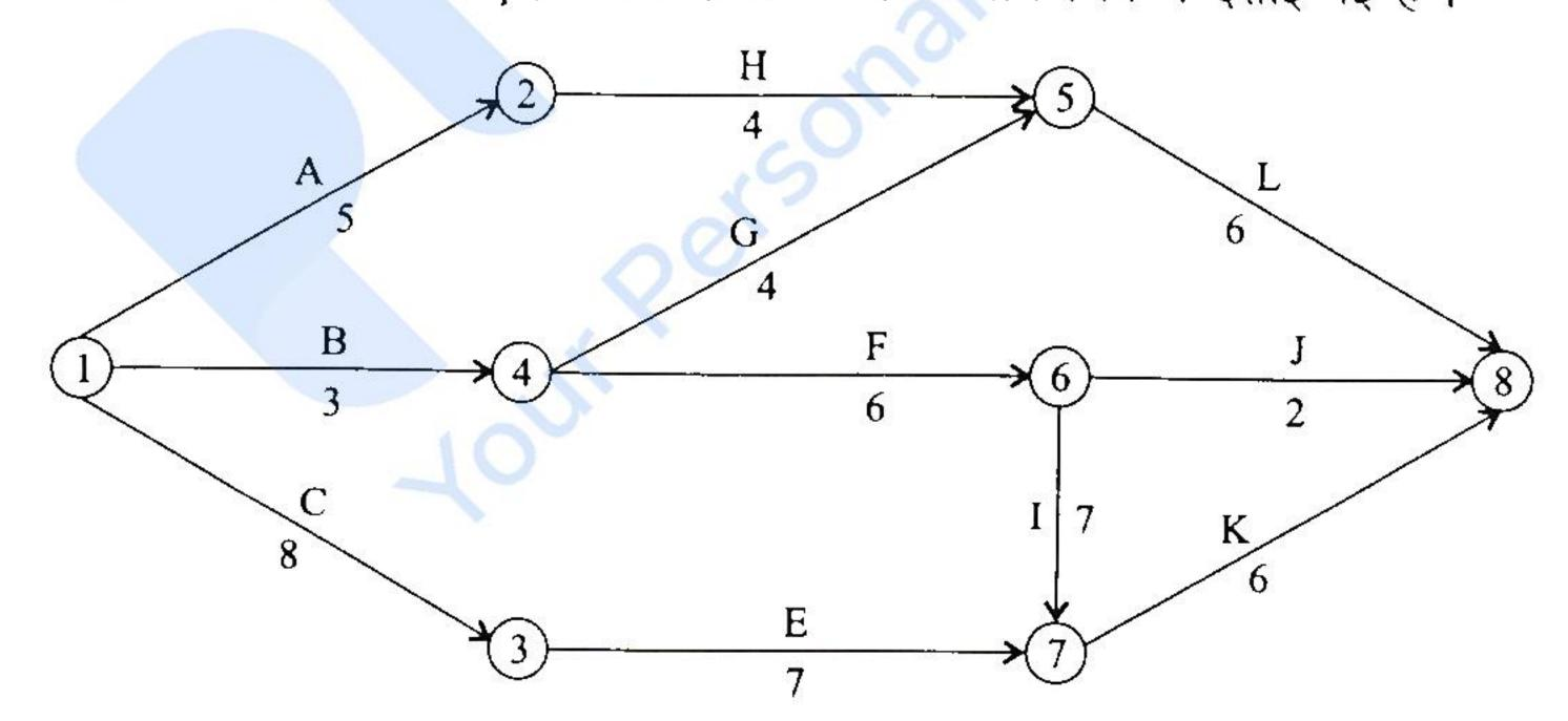
Convert the given A-O-A (Activity on Arrow) to A-O-N (Activity on Node) Network and indicate the critical path. The duration of each activity is shown in the figure. 10
