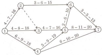
The network for a construction project is shown in the figure given below. The three time estimates for each activity are given along each activity arrow. Determine the:
