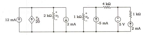
In the circuit given here, find the value of voltage  $v_1$ :
