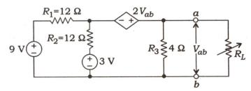
In the circuit diagram given here, load resistance  $R_L$  is to be set for maximum power transfer. Draw Thevenin equivalent circuit across ab and calculate the value of  $R_L$  for maximum power transfer. Also calculate the power loss in resistance  $R_3$ , when the circuit is delivering maximum power to load  $R_L$ :
