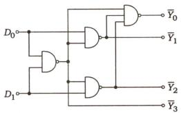
Find the logic equations for the outputs in the concise form and write the corresponding truth table for the circuit given below:
