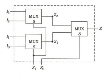
A circuit using three 2-input multiplexers is shown below. Determine the function performed by this circuit :
