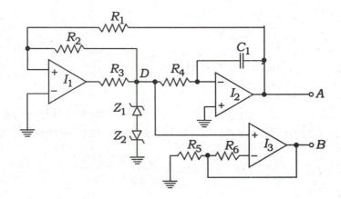
Suggest to replace suitable resistances so that the output voltages at A and B are having swing of  $\pm 6$  V and the output frequency is fixed to 500 Hz.
