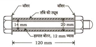
Two thick washers are placed on the two ends of a copper tube and a steel bolt of pitch 1.8 mm is made to pass through these washers as shown in the figure below. The nut is tightened first with hand so that there are no stresses in the tube. Now, the nut is further tightened with the spanner through one-fourth of a turn. Calculate the axial stresses developed in the tube and the bolt. Young's modulus values for steel and copper are 200 GPa and 105 GPa, respectively:
