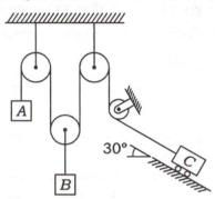
Bodies A, B and C of weights 100 N, 200 N and 150 N, respectively are connected as shown. If released from rest, what would be their respective velocities after 1 s? The pulleys are massless:
